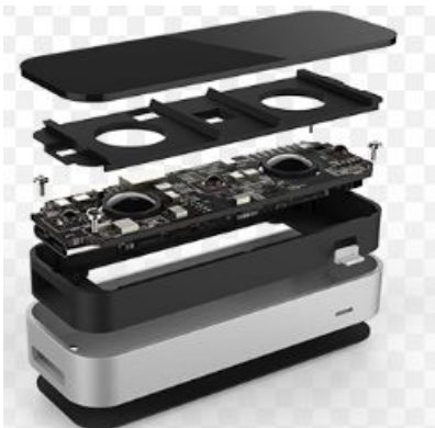
Fig. 2 Inner Parts of Leap Motion Controller
