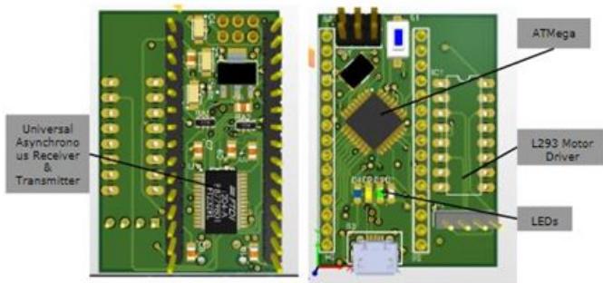
Fig. 10 3D layout view of the Front & Back of the PCB
